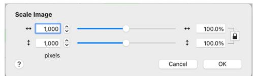
*Note:* The Scale Image function only resizes the whole picture, any selection within the picture is ignored. To resize part of the picture, use the resize handles to resize that selection. See “Select a Block of Objects” on page 20.
